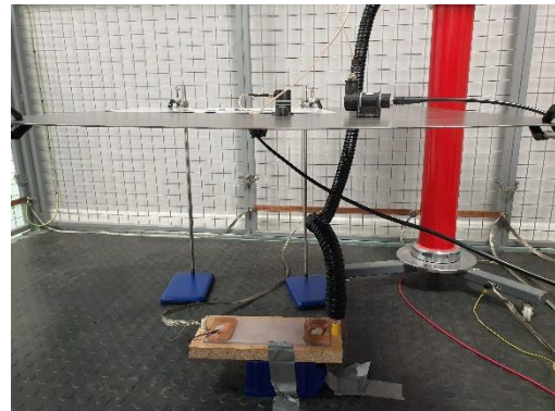
Figure 11. A photo of the experimental setup in the high-voltage test area. Which consists of the contact AE sensor on the top and the AA sensor on the bottom of a 2mm thick steel plate above a surface tracking PD sample.
