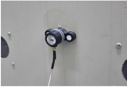
Figure 8. The contact AE sensor is installed externally on the asset of interest with ultrasonic gel between the contact sensor and the asset enclosure.
