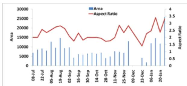
The evolution of the displacement of the hysteresis loop is shown in Figure 10. It can be seen that following the Christmas period of low load (Figure 6) the hysteresis area,
