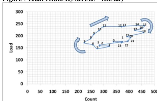
The hysteresis loop has been observed to shift throughout several daily cycles. The direction of movement could be another indicator to monitor the criticality of discharges. Hysteresis loops for four Wednesdays in Jan 2010 are shown in Figure 8. All the loops are generally moving towards the right indicating an increase in the number of discharges and an increased likelihood of failure. There is a decline in the number of discharges on 20th of January which is also seen in Figure 6.
