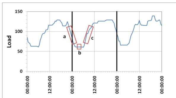
In some cases cable failures have occurred following load increases and in other cases following load a decrease. Determining a measure for the relationship between load and pd is another key factor to take account of in assessing circuit or switchgear criticality.
